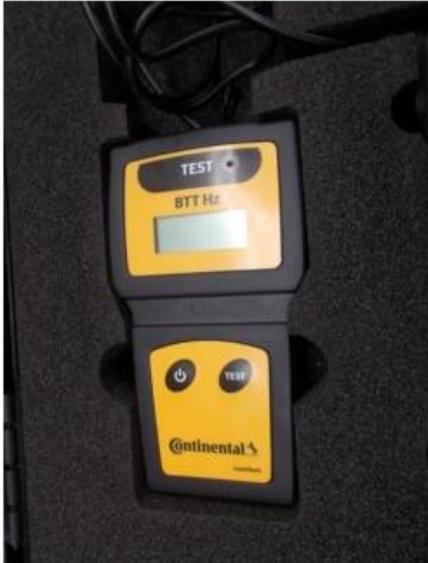
Fig.67 Belt Tension Tester BTT HZ
