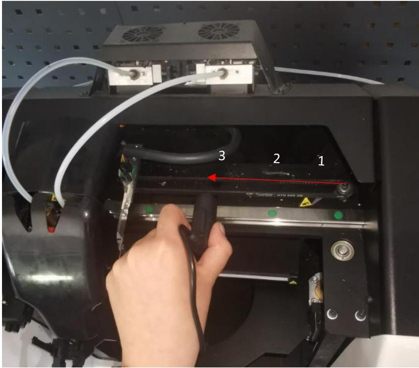
*Fig.69 Measurement toothed belt on the X axis*
