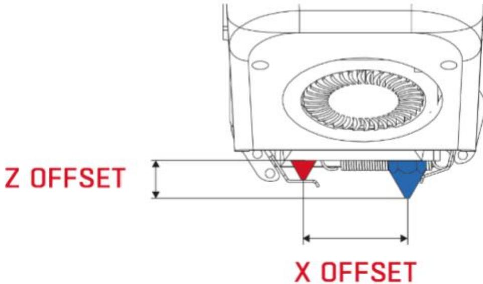
Fig. 61 Visualization of the nozzle position difference (offsets)
