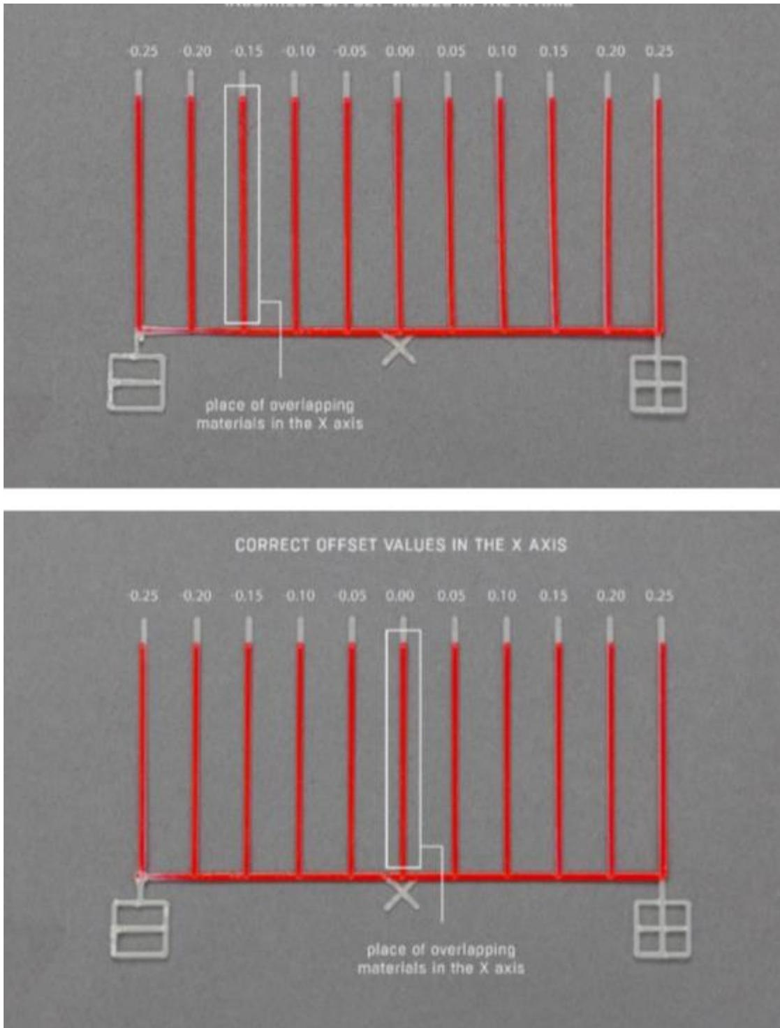
*Fig. 64 Comparison of correctly calibrated offset values with incorrectly calibrated ones*
