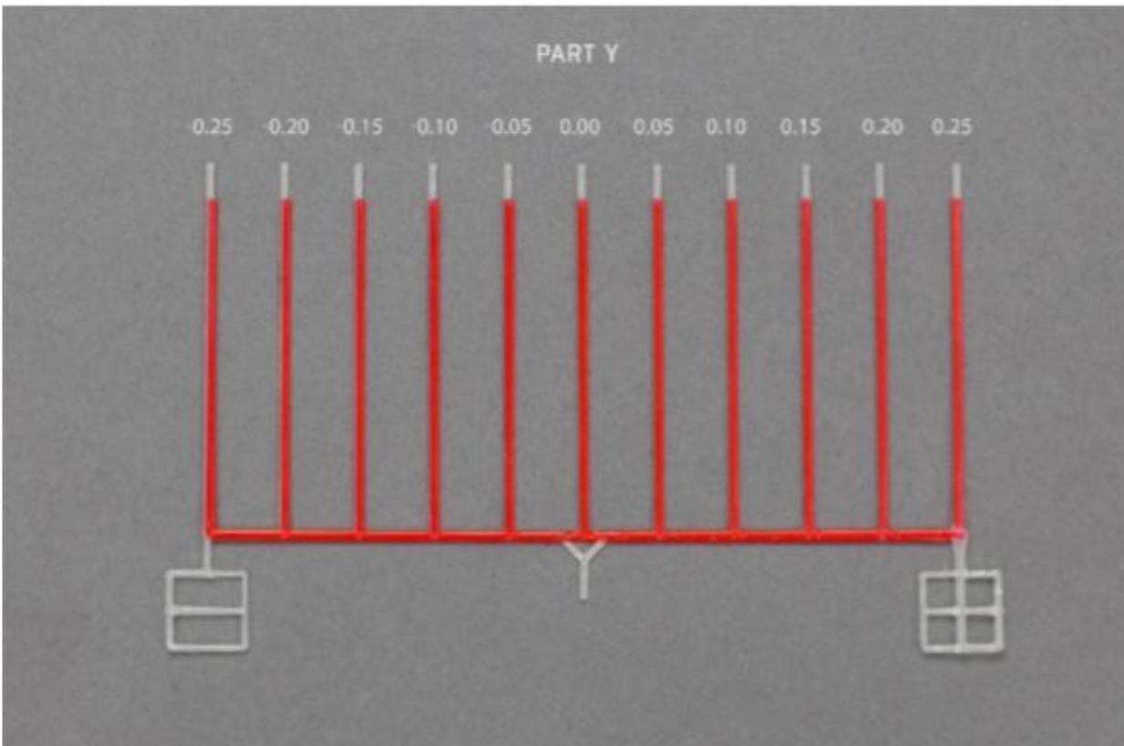
Fig. 63 Calibration model of offset along Y axis
