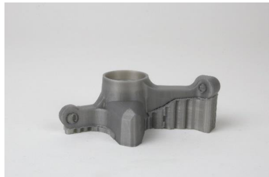
Fig. 2 Model printed from PLA model material and PLA support material
