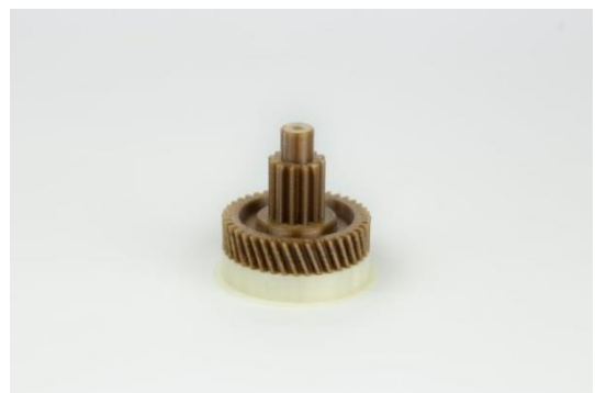
Fig. 4 Model printed from PEEK material model and ESM-10 support material
