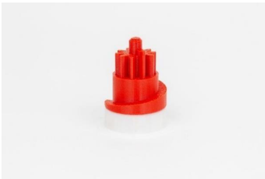
Fig. 1 Model printed from ABS model material and HIPS support material
