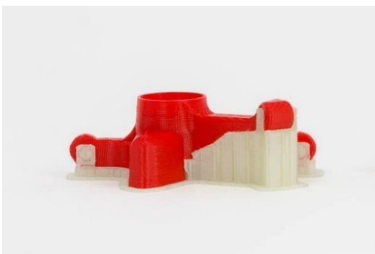
Fig. 3 Model printed from PLA material model and BVOH support material
