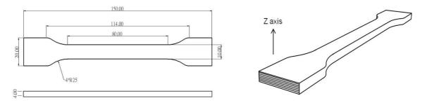
FLEXURAL TESTING SPECIMEN ISO 178, GB/T 9341
