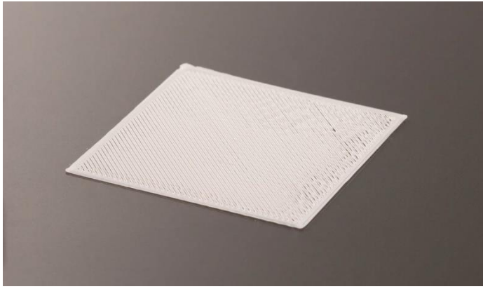
Fig. 36 Example of too low setting of the heatbed
