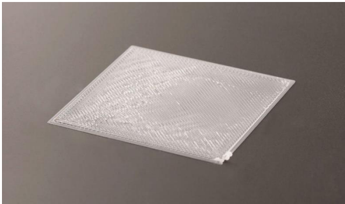
Fig. 34 Example of too high setting of the heatbed
